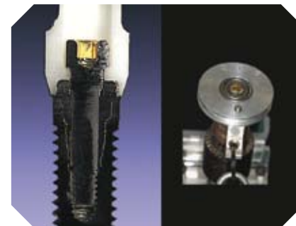
Cross-section of the internal connec- tion implant-ceramic abutment joint and a rotational load fatigue testing jig.
